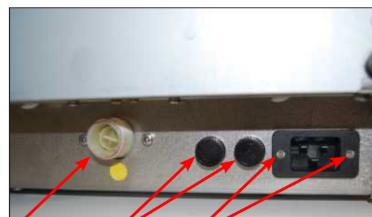
RO valve (if fitted) fuses screws Figure 48
